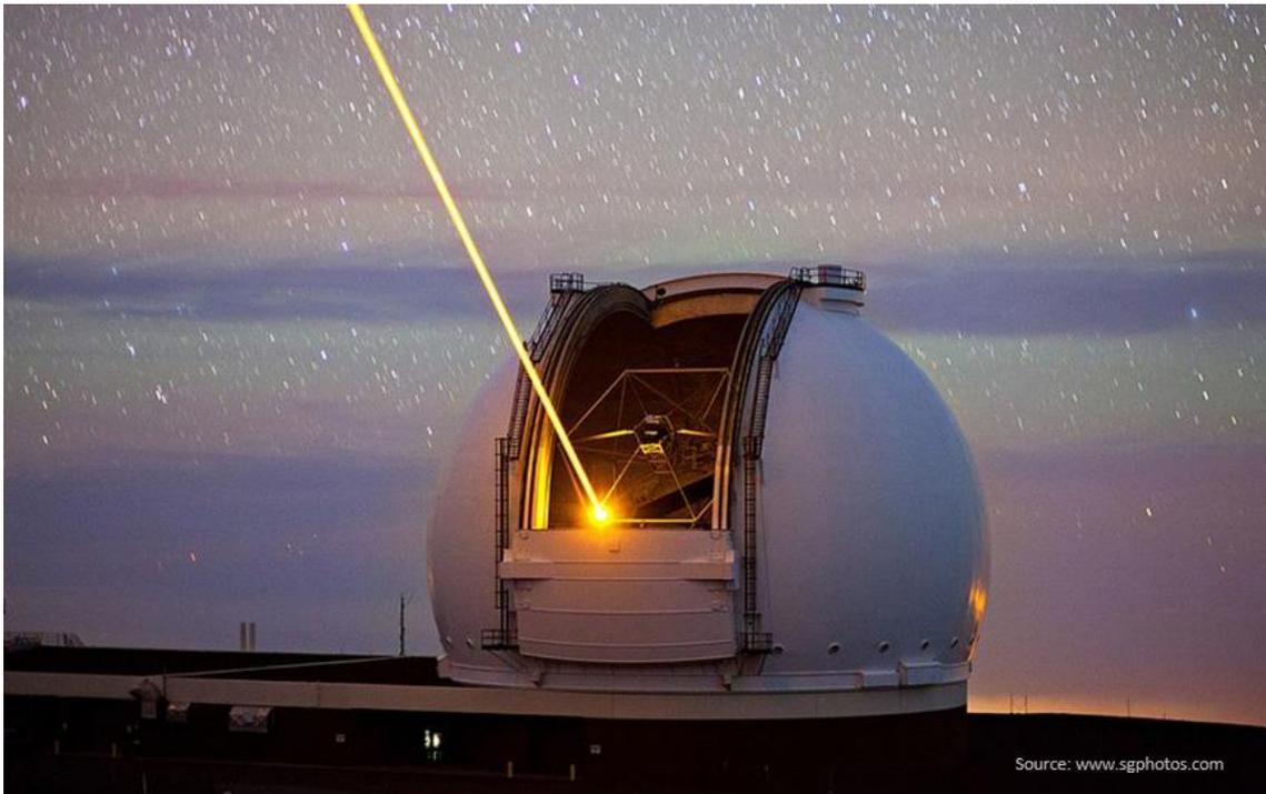
A guide star laser in operation removing atmospheric distortion from star images. The EOS process works in reverse to remove atmospheric distortion from beams transmitted up from the ground.
