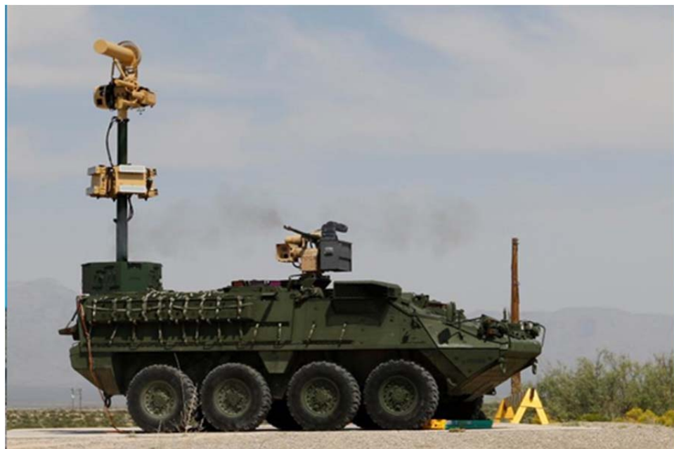
Figure 2: Typical Counter-UAS configuration with EOS weapon system
