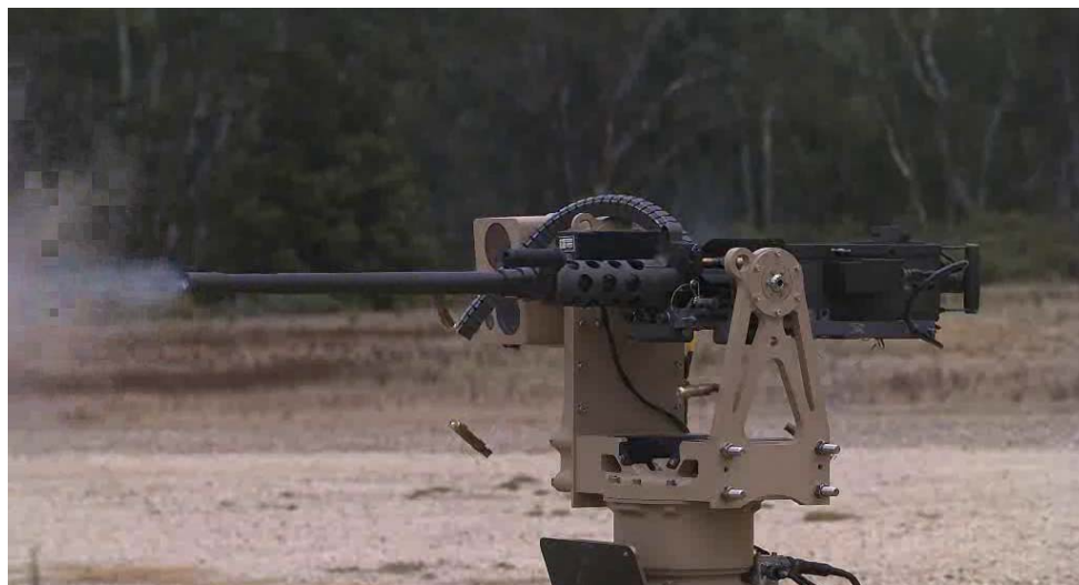
Figure 6: R-150 RWS firing M2 12.7 mm heavy machine gun
