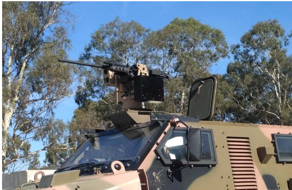
Figure 5: EOS R-150 RWS with M2 12.7 mm heavy machine gun
