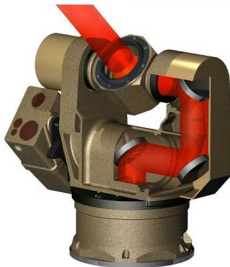
Figure 4: EOS R-600 RWS in directed energy (laser) configuration
