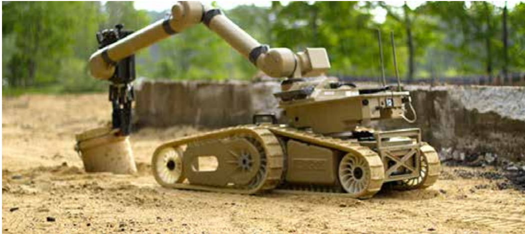
The U.S. iRobot Warrior, using a tool on the end of its arm, is able to grab, lift and carry heavy items. The arm can lift up to 350 pounds and the Warrior can carry a payload of up to 150 pounds. (Photo Credit: Courtesy of iRobot)
