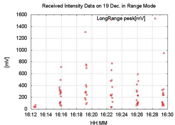
Fig. 2 The laser power equivalent received with LIDAR. The unit of the vertical axis is millivolts, which is the raw telemetry data of peak hold circuit of the received signal strength. Signals are detected in every 3 minutes, because of the range gate, rate of the onboard clock, and the spacecraft motion.
