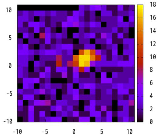
Fig. 1 The number of first pulse detection flag in the transponder mode with respect to the spacecraft scan. Horizontal / vertical axis corresponds to the right ascension / declination direction of the spacecraft attitude. Color shows the number of detection flag. Origin of this figure is the best estimated location of boresight direction before launch. The size of a tile is 1 mrad by 1 mrad.
