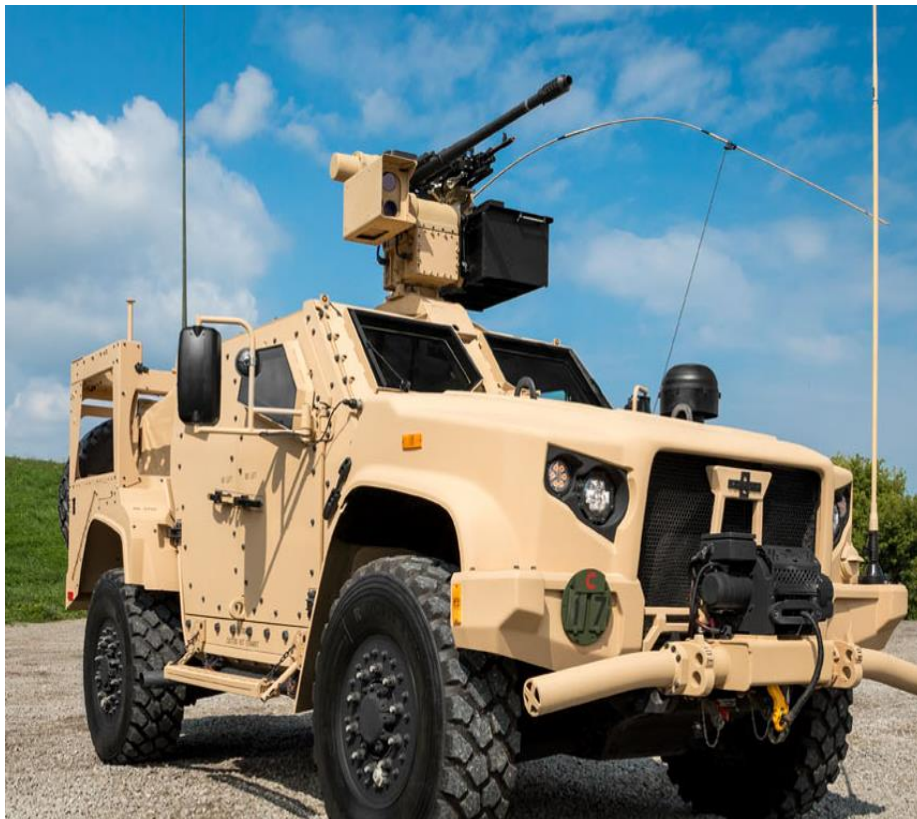
Photo: The new EOS 30mm remote weapon system integrated with the U.S. Army JLTV
